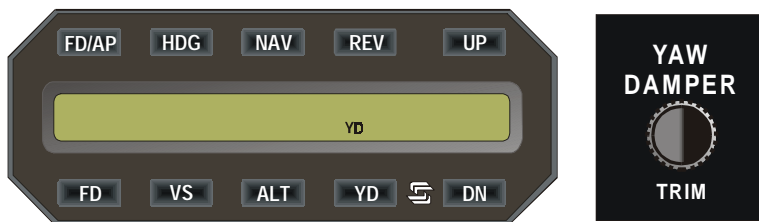
Fig. 4-13 Yaw Damper Controls
