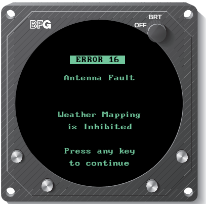
Figure 3-11. Error Message for a Recoverable Weather Fault
