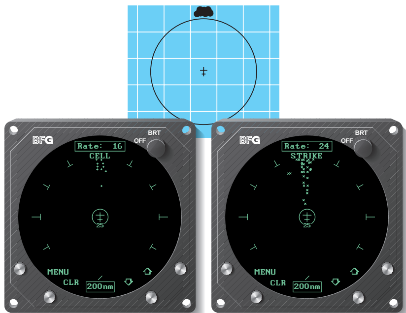
Figure 4-11. Discharge Points Off Aircraft's Nose
