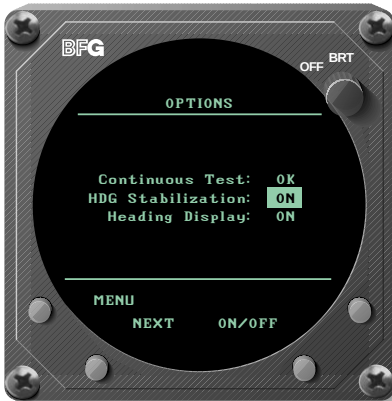
Figure A-3. OPTIONS Screen With Heading Stabilization
