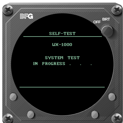
Figure 3-2. System Test in Progress
