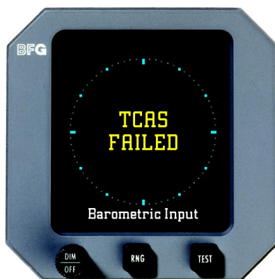
Figure 2-12. TCAS Failed/Barometric Input Screen
