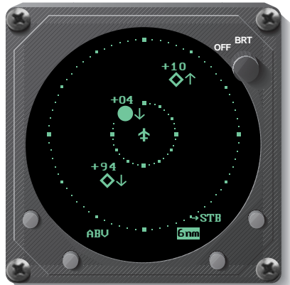
Figure 3-6. Traffic Screen on the Ground
