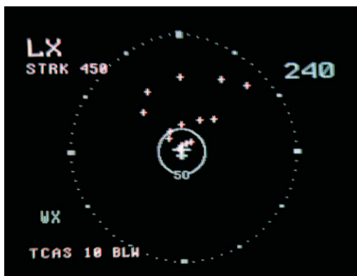
Figure 3-3. 360° View Lightning Screen
