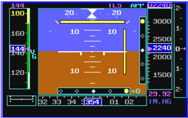
In approach mode, the vertical and horizontal guidance needles turn yellow when full needle deflection is detected on the ILS.
