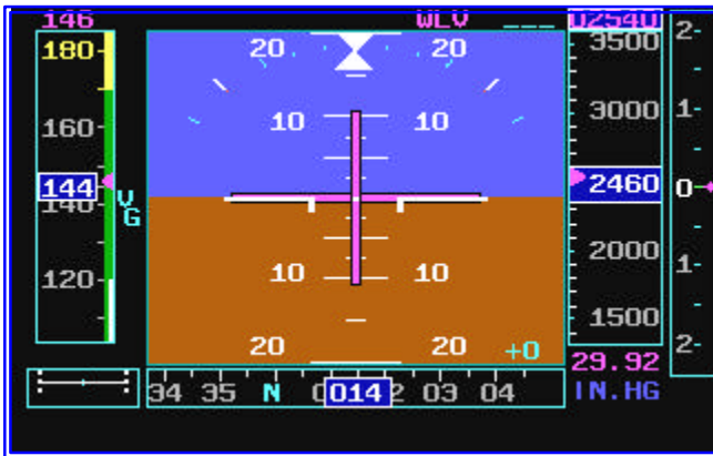
Flight Director engaged in Wing Level “WLV” mode
