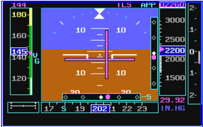
Flight Director engaged, “ILS” and “APP” annunciators on the upper right side of the EADI.
